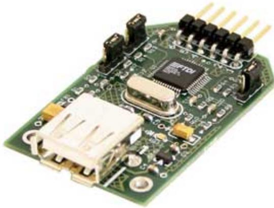
to be connected to it. Using the Vinculum VDIF firmware the VNC1L-1A's I/O interface can be selected between the serial UART or SPI using the on-board jumper pins. VDRIVE1 is designed for evaluation and development of VNC1L-1A applications. With its attractive quantity discount structure, VDRIVE1 module is also suitable for incorporation into finished product designs.
