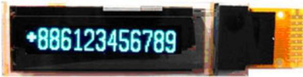
Univision, available through [GLYN High-Tech Distribution](#), has introduced a new low cost, 0.85" diagonal screen size, monochrome (light blue) OLED module (part number UG-0416ALBAG01). With a
