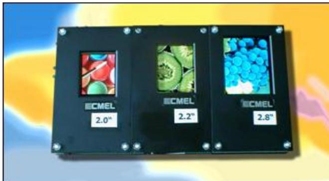
OLED (Organic Light-Emitting Diode) is a self light-emitting technology composed of a thin, multi-layered organic film placed between an anode and cathode. In contrast to LCD technology, OLED does not require a backlight. OLED possesses high application potential for virtually all types of displays and is regarded as the ultimate technology for the next generation of flat-panel displays.
