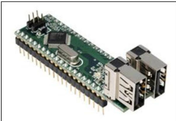
FTDI, available through [GLYN High-Tech Distribution](#), has released a new version of the VDIP module with two USB connectors to allow for easier prototyping of applications requiring two full-speed USB host/slave interfaces.
