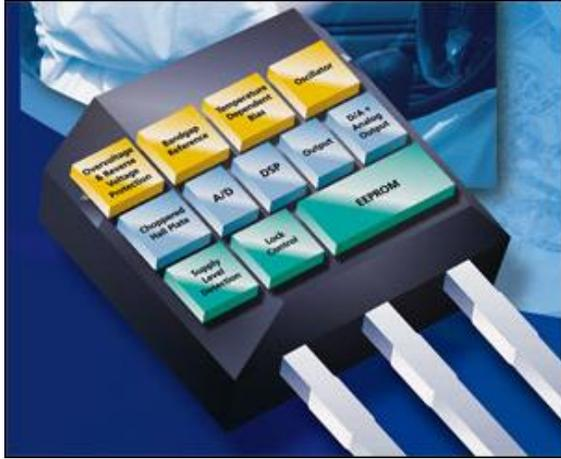
Like its predecessors of the second generation, the HAL 82x has an integrated EEPROM to store the sensor parameters. Proven in previous generations of Micronas Hall-effect sensors, the EEPROM is extremely robust and reliable, even at the allowed maximum junction temperature of 170 °C.
