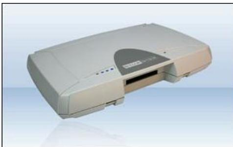
WRAP Access Server™ is targeted at system integrators and original equipment manufacturers wanting to deploy a secure, cost effective, low power consuming and up to 100-meter range wireless network for Bluetooth-equipped devices. These devices include products such as barcode readers, pay-terminals, medical instruments, special purpose PDAs and mobile phones, and telemetry and machine-to-machine units.
